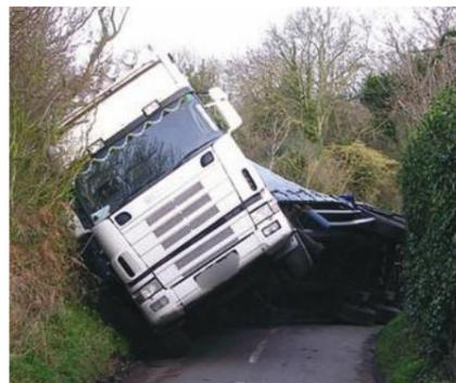
Operators will need to pay particular attention to curtain-sided trailers. VOSA's advice to industry is that curtain-sides should not be thought of as a restraint system. Loads carried in curtain-sided vehicles should be secured appropriately, without using the curtains as part of the securing system.
